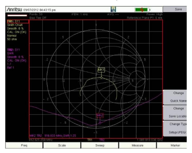
To see if these slight differences would cause a problem, I took an antenna that was very poorly matched, measured S11 on both VNAs, and added components of a pi-matching network one at a time, measuring with both VNAs after adding each component. It's hard to know because it wasn't a blind experiment because I saw both sets of results. My gut feeling is that Anritsu is more accurate but I could match an antenna on the VIA Echo as well as on the Anritsu.
