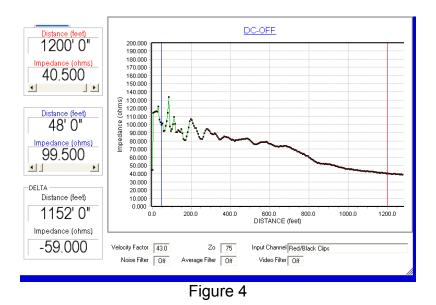
Figure 4 shows a large gauge cable. Ignoring the spikes caused by connected electronic packages, this twisted pair cable appears to loose about 60  $\Omega$  over 1152 feet (351m) as marked by the blue and red cursors.
