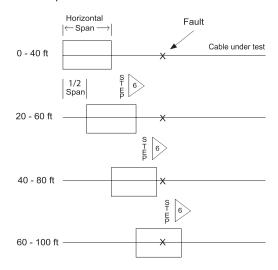
Setting the Start Distance of the plot using the STEP key.
