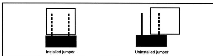
**Figure 5 - SWR-121 V/U Jumper Installation/Removal**
