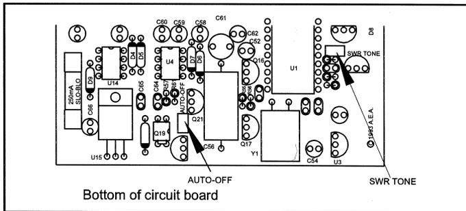
Figure 4. SWR-121 V/U Jumper Locations
