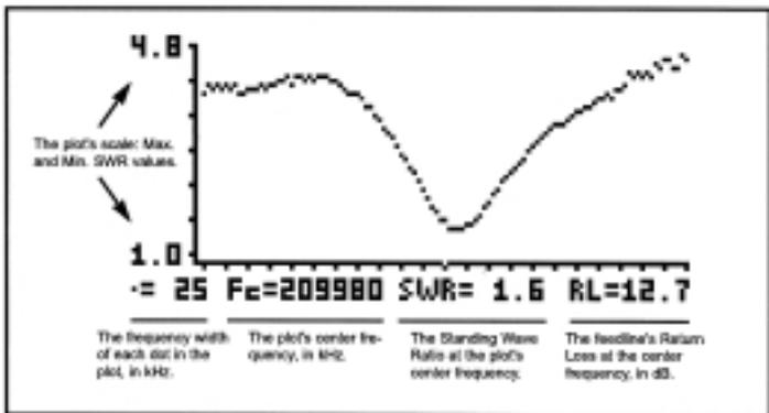
Figure 1 - SWR-121 V/U Display
